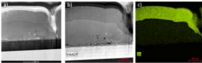
Figure 6: a) BF image of the cross-section of a CZTSe solar cell with reduced number of secondary phases. b) HAADF of the same area and c) EDS mapping of Zn showing no segregation.
