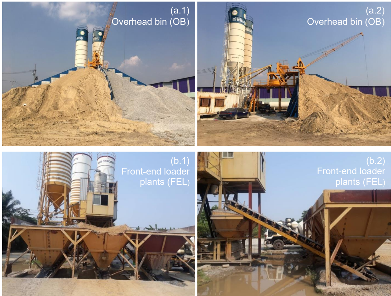
Fig. 1 (a) Aggregate unloading to OB plant and (b) aggregate feeding in FEL plant.
